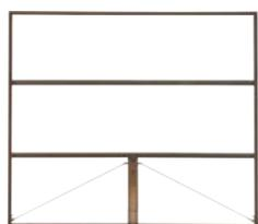
The OFI is an open frame ready to take your own design of infill. Maximum infill weights of 7kgm<sup>2</sup> for 1,981mm (6'6") high doors and 10kgm<sup>2</sup> for 2,134mm (7'0") high doors. Maximum timber infill thickness = 18mm.
